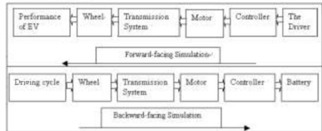
Fig. 2. Schematic showing forward-facing and backward-facing simulation methodologies [8]
