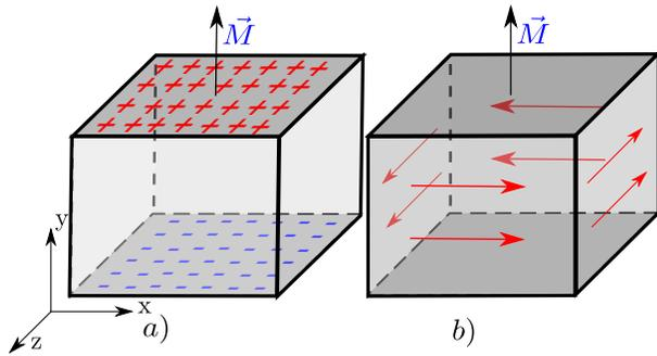
Fig. 6. Explicative to equivalent charge a), and current sheets b).
