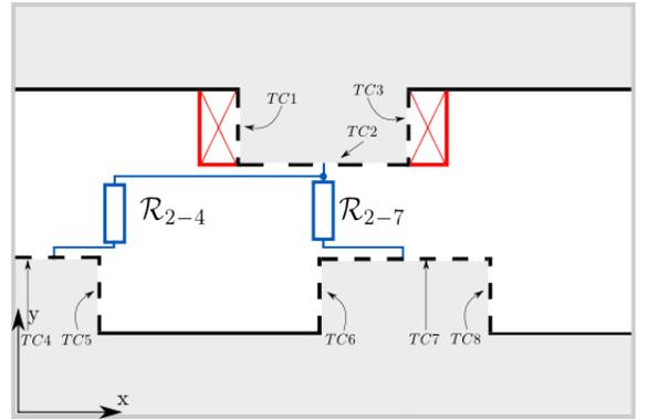
Fig. 3. Example of reluctance network for tooth contour method
