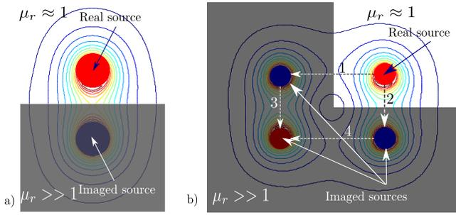
Fig. 7. Explicative to Method of images: a) Flat boundary b) Right angle boundary.
