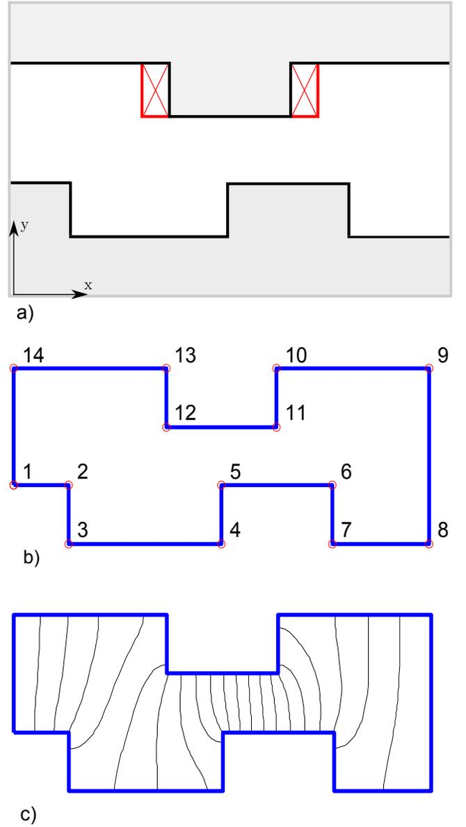
Fig. 4. Schwartz - Christoffel mapping for slotted structure, a) The slotted structure geometry in polar coordinates, b) Equivalent polygon ready to be mapped, c) Result of SC mapping from a rectangular shape
