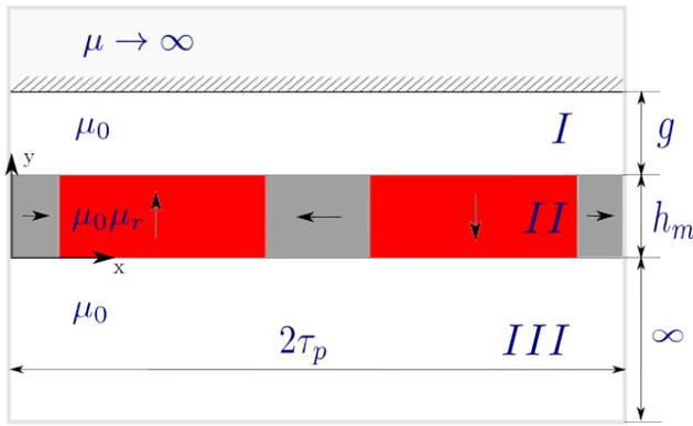
Fig. 5. Linear Actuator Topology adopted for Harmonic Model
