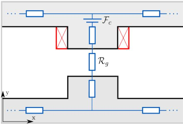
Fig. 2. Example of magnetic equivalent circuit
