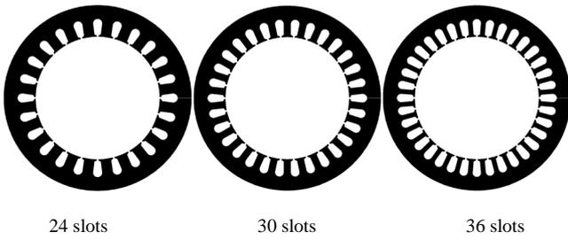
Fig. 3. SynRM stator structures
