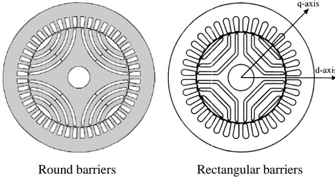
Fig. 4. Typical flux barrier shapes
