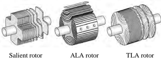
Fig. 1. Synchronous Reluctance Motor rotor types [9]
