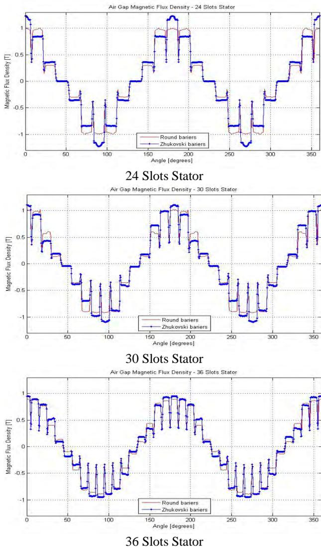
Fig. 7. Air gap magnetic flux density repartition
