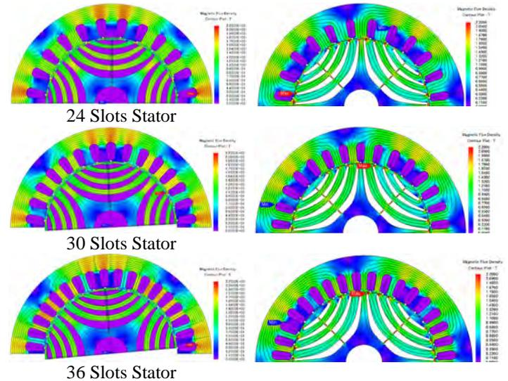
Fig. 6. Magnetic flux density and flux lines
