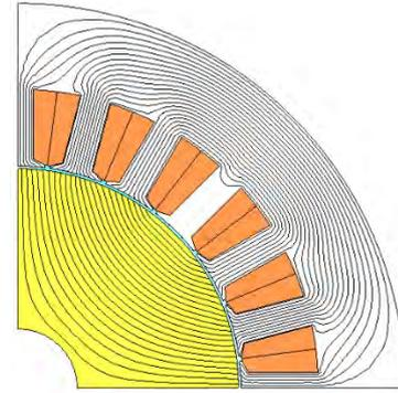
Fig. 5. Natural flux lines in machine with solid rotor
