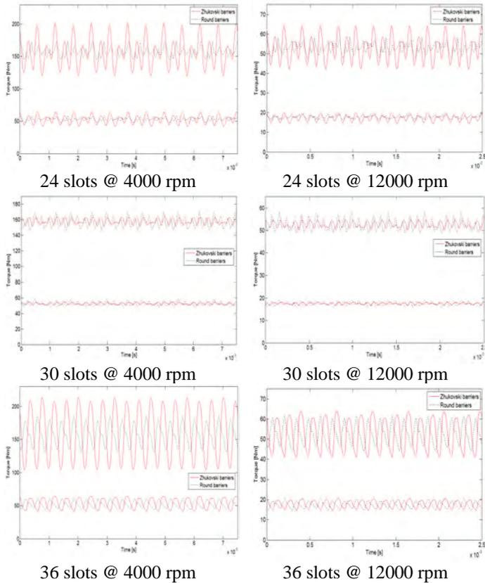
Fig. 10. Torque comparison of instantaneous torque of all machine topologies
