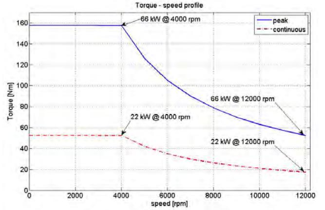
Fig. 2. Torque/speed profile for peak and continuous power
