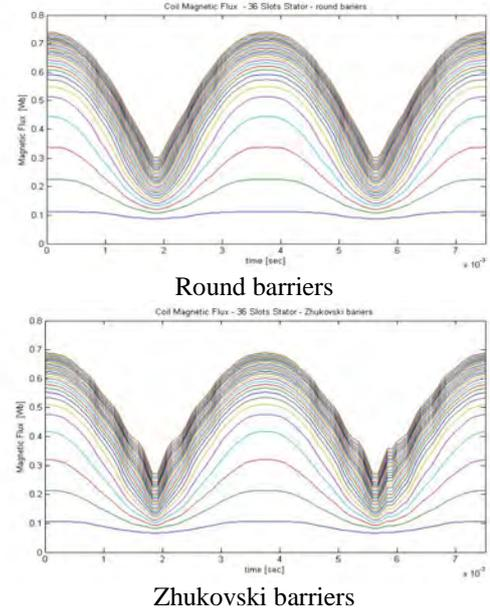
Fig. 8. Coil magnetic flux variation
