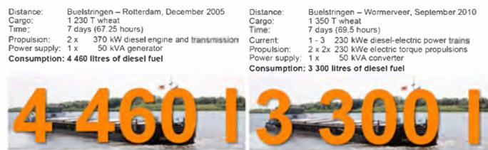
Fig. 3. Illustrating 25% diesel fuel savings for 1 week of shipping on a specific journey [12].
