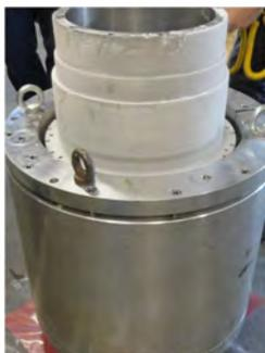
Fig. 13 Rotor shaft with lamination stack and magnets showing mounting tooling.
