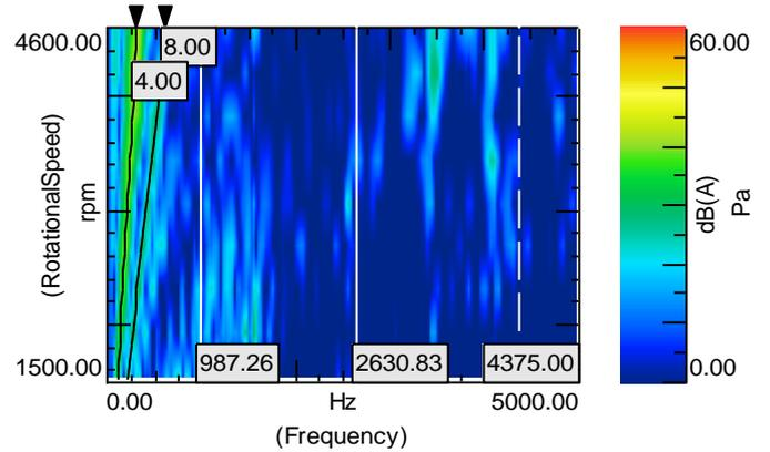
Figure 7. Acoustic pressure dB (RMS) A for the first rotor topology – frequency range 5000 Hz
