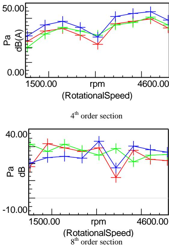
Figure 9. Order cut for the first (red) second (green) and third (blue) rotor topology – frequency range 2000 Hz
