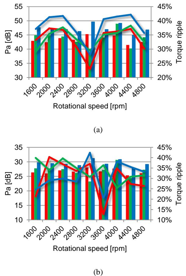
Figure 10. Order cut (lines) for 4<sup>th</sup> (a) and 8<sup>th</sup> (b) orders and torque ripple (columns) for the first (red) second (green) and third (blue) rotor topology
