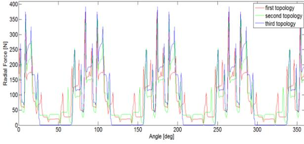
Figure 5. Radial forces for the first (red), the second (green) and the third (blue) rotor topology at 4400 rpm
