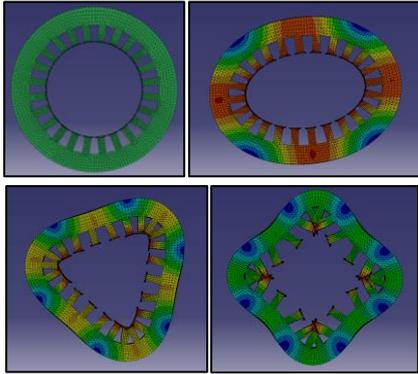
Figure 6. Structural mesh, Ovalization mode (985 Hz), Triangular mode (2559 Hz) and Square mode (4375Hz) of the stator
