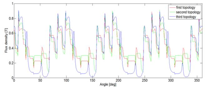
**Figure 3. Air gap magnetic flux density along rotor's periphery for the first (red), the second (green) and the third (blue) rotor topology**
