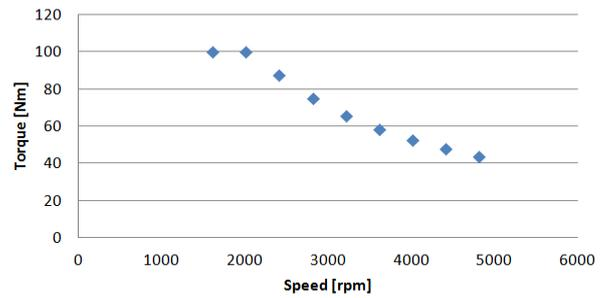
**Figure 2. Torque vs. speed curve of analyzed motor**
