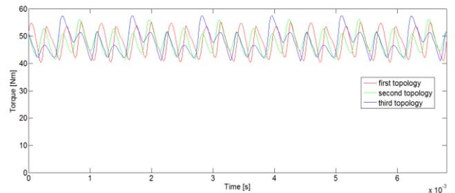
**Figure 4. Output torque function of time for the first (red), the second (green) and the third (blue) rotor topology at 4400 rpm**
