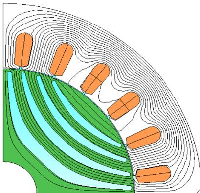
Fig. 6. One pole of the machine with flux lines: machine with Zhukovski type barriers in the rotor
