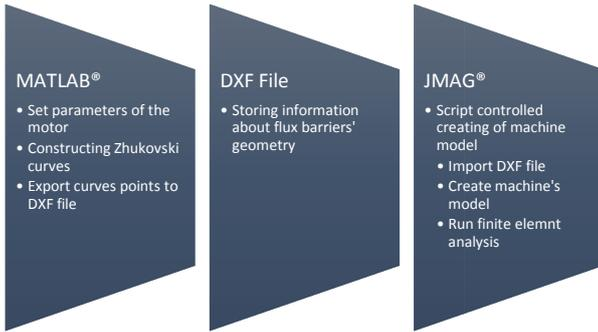
Fig. 5. Process of machine's model development
