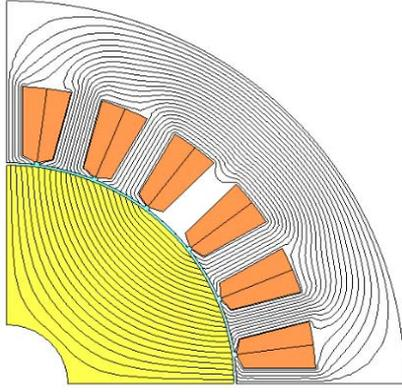
Fig. 2. Natural flux lines in machine with no flux barriers in the rotor
