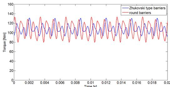
Fig. 10. Torque comparison: machine with Zhukovski's curve based flux barriers (blue) and machine with round flux barriers (red)
