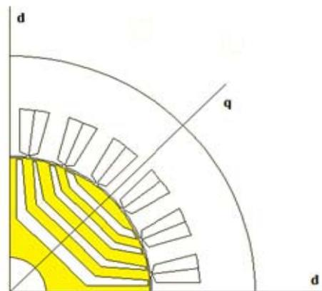
Fig. 1. One pole of synchronous reluctance machine with four flux barriers in the rotor.
