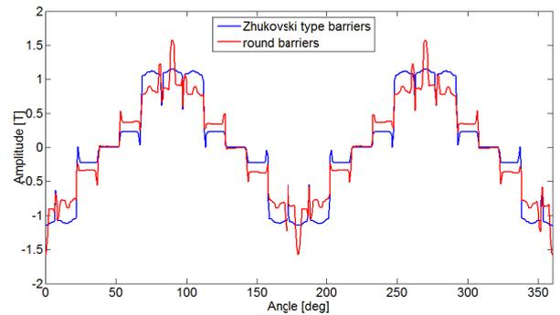
Fig. 8. Radial components of air gap magnetic flux density: machine with round flux barriers (blue) and machine with Zhukovski's curve based flux barriers (red)
