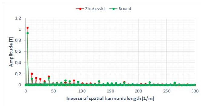
Fig. 9. FFT of air gap magnetic flux density: machine with Zhukovski flux barriers (blue) and machine with round barriers (green)
