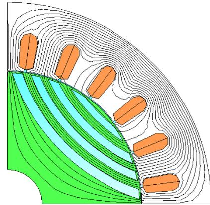
Fig. 7. One pole of the machine with flux lines: machine with round barriers in the rotor
