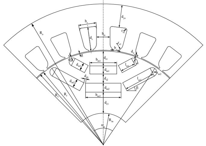
Fig. 2. IPM motor topology with geometric design parameters
