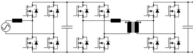
Fig. 12. Single-stage, single-phase, bidirectional, isolated, soft-switched AC–DC converter based on the full-bridge full-bridge DAB.
