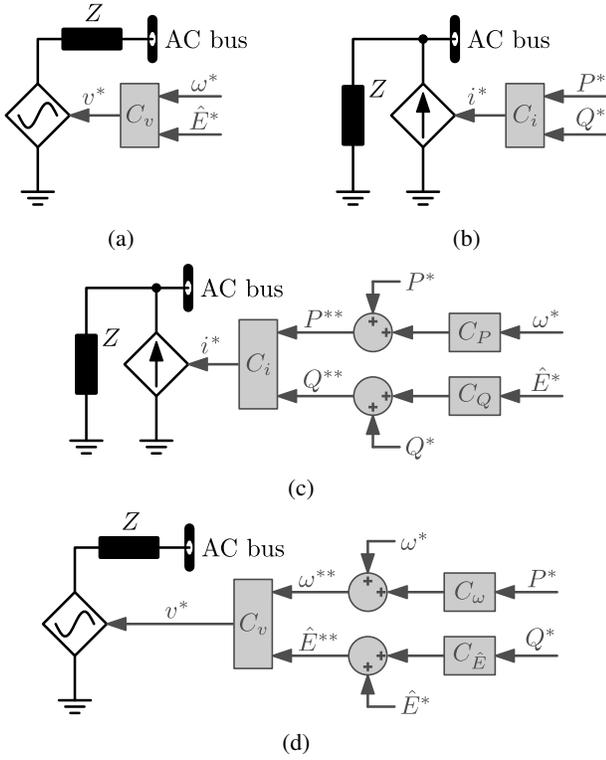
Fig. 3. Simplified representation of grid-connected power converters [9]. (a) Grid-forming, (b) grid-feeding, (c) grid-supporting (current-source-based), and (d) grid-supporting (voltage-source-based).
