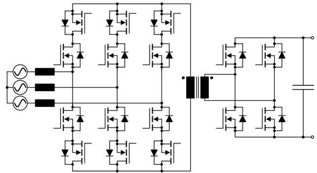
Fig. 14. Single-stage, three-phase, bidirectional, isolated, soft-switched AC–DC converter, using a cycloconverter on the AC side, a voltage-source converter on the DC side, and a medium frequency transformer in between.
