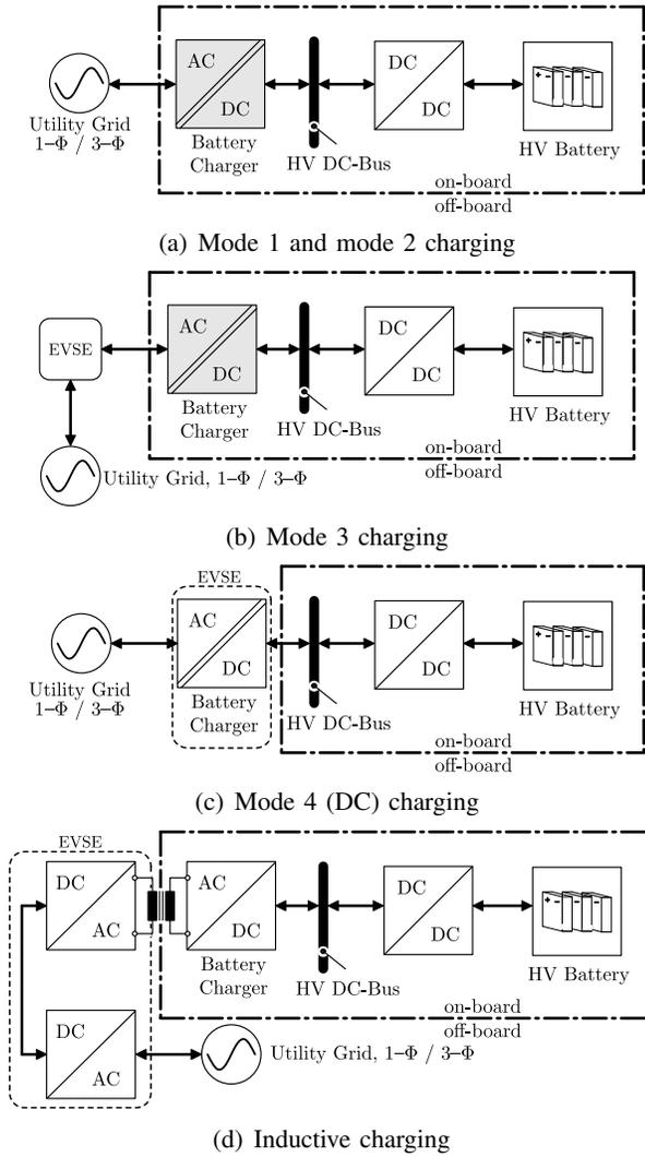
Fig. 2. Charging infrastructure for conductive (a)-(c) and inductive (d) charging. Note that the DC output of the battery chargers might also be directly connected to the terminals of the HV battery.
