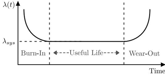
Fig. 6. A typical reliability curve (also known as Bathhtub curve), indicating the failure rate of a device during different time intervals of its lifetime.
