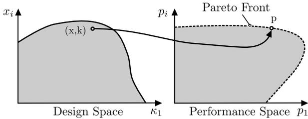
Fig. 7. Qualitative representation of the Design Space (left) and Performance Space (right), illustrating a random mapping of a design decision  $(x,k)$  to the corresponding performance. The boundary of the Performance Space is defined by the Pareto front which represents the best possible performance of the power electronics system.
