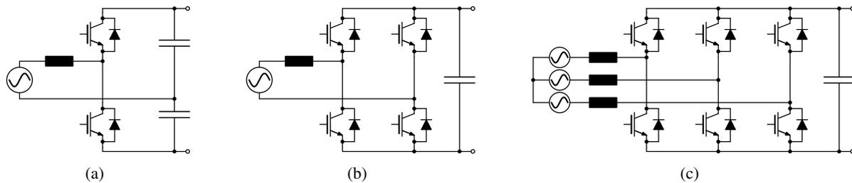
Fig. 9. Bidirectional PFC AC–DC converter topologies based on conventional bridge circuits. (a) Single-phase half-bridge converter, (b) single-phase full-bridge converter, and (c) three-phase full-bridge converter.
