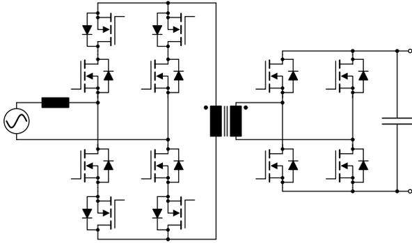
Fig. 13. Single-stage, single-phase, bidirectional, isolated, soft-switched AC–DC converter, using a cycloconverter on the AC side, a voltage-source converter on the DC side, and a medium frequency transformer in between.
