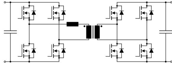
Fig. 11. Isolated, bidirectional, full-bridge full-bridge DAB DC–DC converter.
