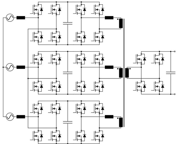
Fig. 15. Single-stage, three-phase, bidirectional, isolated, soft-switched AC–DC converter based on separate single-phase matrix-type ‘low-frequency AC to high-frequency AC’ modules using a single transformer structure.
