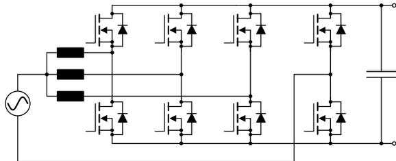
Fig. 10. Single-phase, bidirectional, multi-cell, totem-pole PFC AC–DC converter.
