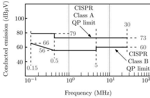
Fig. 4. Quasi-peak limits for conducted emissions at the main ports of Class A and Class B equipment according to CISPR 11 and 22.
