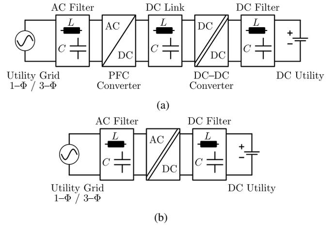
Fig. 8. General representation of (a) dual-stage AC–DC converter topologies and (b) single-stage AC–DC converter topologies.
