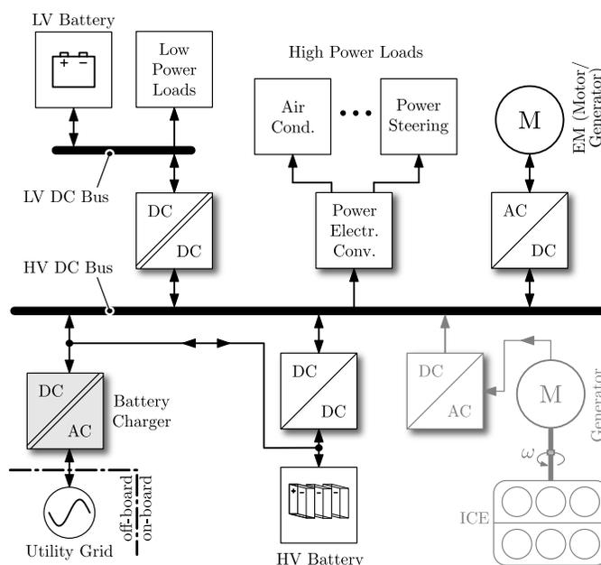
Fig. 1. Typical PBEV electric power system architecture [3]. The PBEV turns into a PHEV in case an internal combustion engine present (gray colored part).
