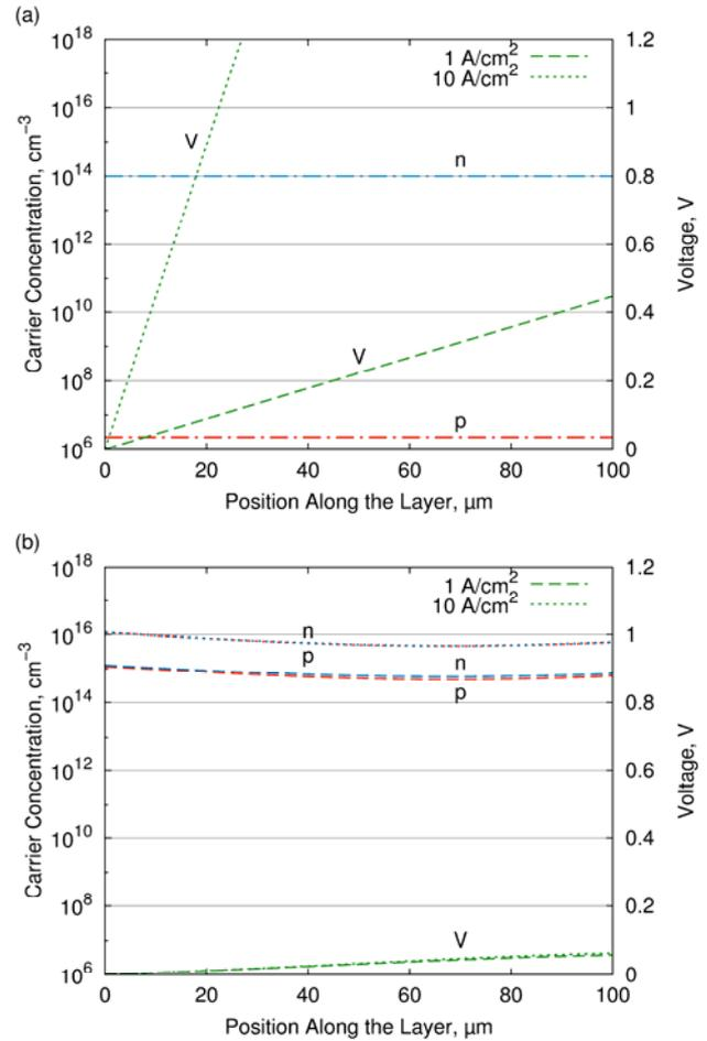
Fig. 2: Electron concentration  $n$ , hole concentration  $p$  and voltage drop  $V$  along a lightly doped n-type semiconductor layer ( $W = 100 \mu\text{m}$ ,  $N = 10^{14} \text{ cm}^{-3}$ ) for two current density values: (a) unipolar conduction, (b) bipolar conduction
