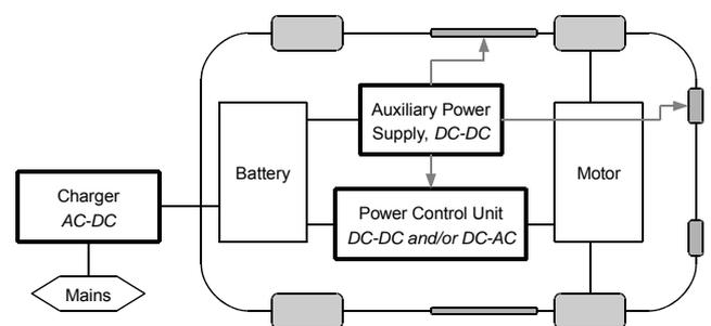
Fig. 4: Fields of SiC application in electric vehicles
