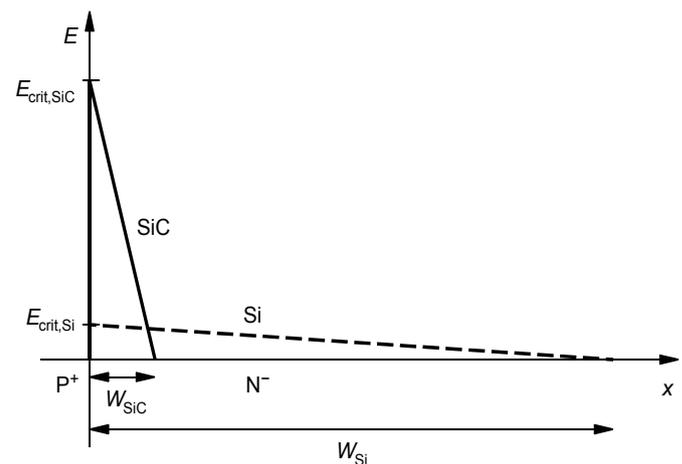
Fig. 1: Electric field distribution at a reverse-biased PN junction in a silicon (Si) and a silicon carbide (SiC) high-voltage power semiconductor device having the same voltage blocking capability
