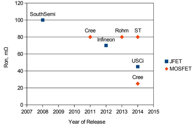
Fig. 3: Commercial silicon carbide transistor technology evolution [24-28]
